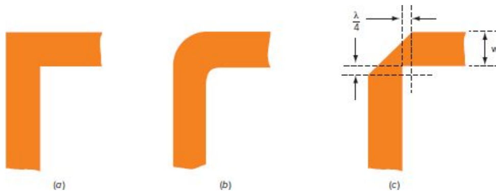
Figure 18-12 Microstrip 90^\circ turns. (a) Right angles such as this should be avoided. (b) Gradual curves or turns are preferred. (c) This arrangement is also acceptable.
