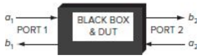
Figure 23-15 Treating circuits and devices as a “black box” two-port network for five-parameter analysis.
