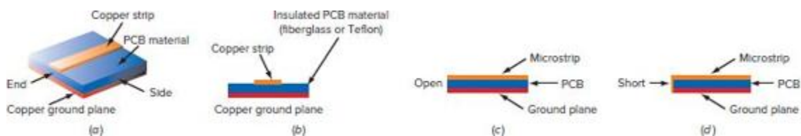
Figure 18-7 Microstrip transmission line used for reactive circuits. (a) Perspective view. (b) Edge or end view. (c) Side view (open line). (d) Side view (shorted line).
