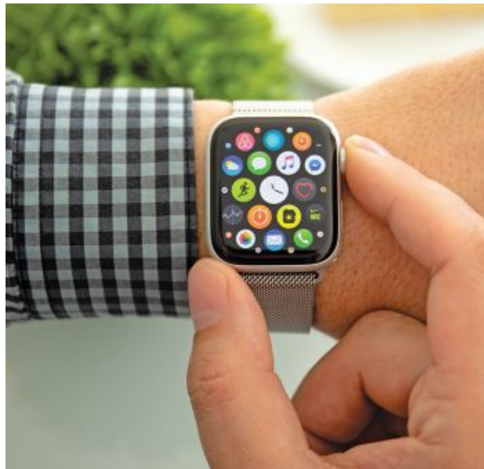
Figure 21-5 The Apple watch communicates with a smartphone with Bluetooth wireless technology.
